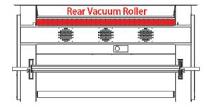
Once the film is detected by the rear sensor, the front vacuum roller will stop suction but continue to transport the film, while the rear vacuum roller will maintain both suction and transport functions.
