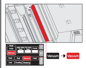
Adjust the position of the powder holders With the media holders pushed close to the media, this ensures Minimal powder will fall outside or off the film, reducing the interval for replenishing powder.
