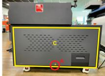
Proceed to remove the side panel from the opposite side, by removing the screw (B).
