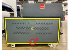
Once both sides are removed, remove the two screws that are holding the hood cover in place. There is one screw either side located as below.
