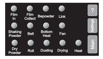
The displayed parameters here correspond to the working status of their respective names and do not support manual adjustment.
