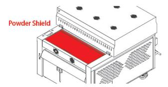
The powder shield's function is to prevent powder from splashing. If it is opened while the machine is running, the powder shaking function will stop. Once it is closed, the powder shaking function will resume.
