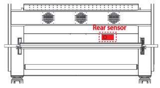
After the transfer film is finished baking, it will exit the oven. The rear sensor is used to detect whether the transfer film has completed baking and emerged from the back.
